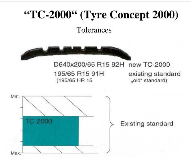
Double Marking (DM) should be possible, if the new tolerances are inside the existing tolerances; DM was possible from "HR" to "R...H"!
