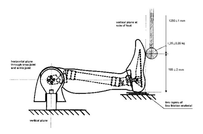
$\frac{\text{Figure 2}}{\text{Lower foot impact test (without shoe)}}$  Test set-up specifications
