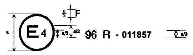
The above approval mark affixed to an engine shows that the engine type concerned has been approved in the Netherlands (E4) pursuant to Regulation No. 96 (according to the level corresponding to power band F) and under approval number 011857. The first two digits of the approval number indicate that Regulation No. 96 was in its amended form (01 series of amendments) when the approval was granted.
