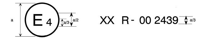
The above approval mark affixed to a pneumatic tyre shows that the type of tyre concerned has been approved in the Netherlands (E 4) pursuant to Regulation No. XX under approval number 002439. The first two digits of the approval number indicate that the approval was granted in accordance with the requirements of Regulation No. XX in its original form.
