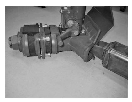
Clarified dimensioning of the D50-X shank would ensure the compatibility with the C50 couplings. See examples:
