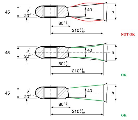
Transitional provisions for the 02 series of amendments are proposed. The new 02 series of amendments would only be mandatory for D50-X drawbar eyes.
