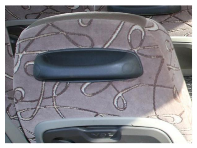
UN Regulation No 80 in force requires dynamic test according to Appendix 1 Test 2 or Appendix 6 pendulum test to show a conformity of back of a seat. In the Appendix 6, which is linked to UN Regulation No 21, point of impact of the pendulum is not clearly defined. That may cause a situation in which the safety of the handle similar to the one shown in picture is not assessed.
