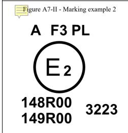
The lamp bearing the approval mark shown on the left is a combination of a front position lamp (A) and a front fog lamp (F3) with a plastic lens (PL) approved in France (E2), under approval number 3223 pursuant to this Regulation (148R) and the UN Regulation for Road Illumination Devices (149R).
