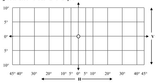
Minimum values: 0.6 cd at any point other than the reference axis, at which it shall be 4.0 cd Maximum values: 25.0 cd at any point
