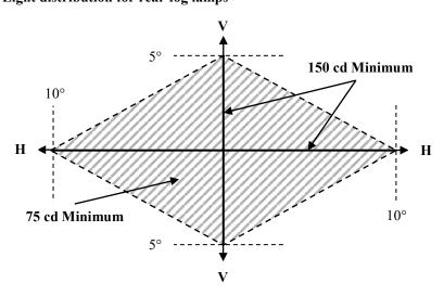
If visual examination of a light appears to reveal substantial local variations of intensity, a check shall be made to ensure that, outside the axes, no intensity
