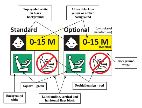
Integral Enhanced Child Restraint Systems that can be used forward facing only shall have the following label permanently attached on the part hosting the child and visible to the person installing an Enhanced Child Restraint System in the vehicle:
