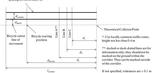
Figure 2: Static Tests
