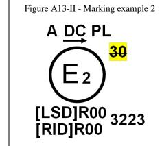
The lamp bearing the approval mark shown on the left is a gas-discharge **passing beam** headlamp (DC) for left-hand traffic only (arrow) using a plastic lens (PL) approved in France (E2) pursuant to this Regulation ([RID]R) as set in the original series of amendments (00) combined with a front position lamp (A) as set in the original series of amendments (00) of the Regulation on Light Signalling Devices ([LSD]R). Both lamps (functions) are approved under approval number 3223.
