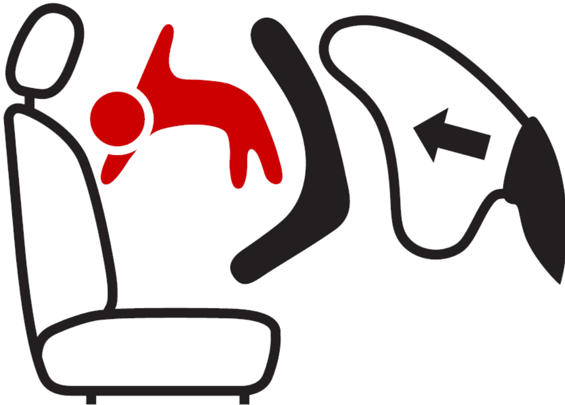
Figure 3 Pictogram depicting airbag deployment danger that shall be used and that shall measure 40 mm in width and 28 mm in height or proportionally larger
