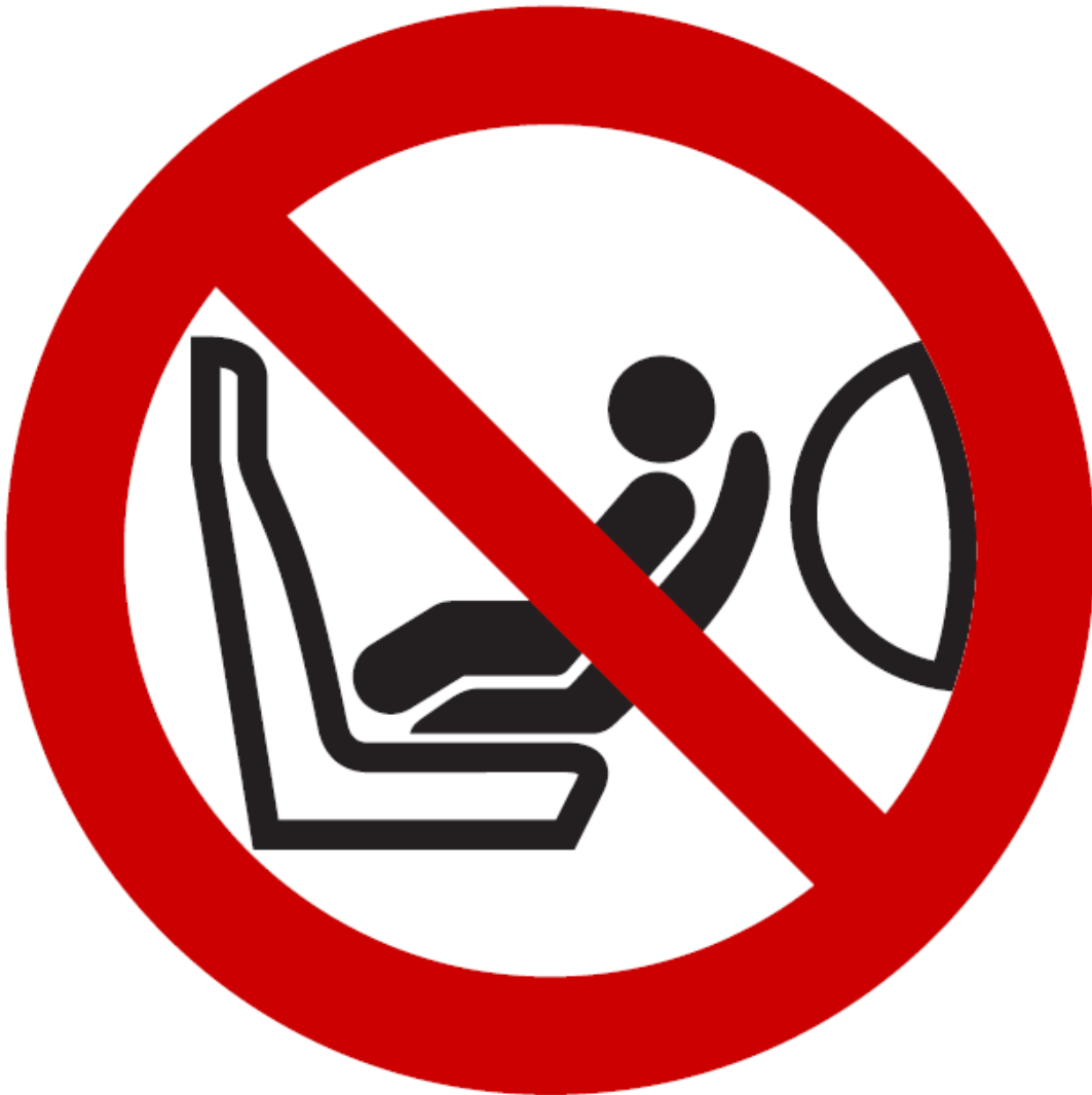
Figure 2 Pictogram according to ISO 2575:2004 - Z.01 that shall be used and that shall have an outer diameter of at least 38 mm
