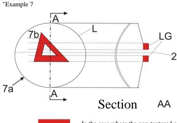
In the case where the non-textured outer lens is excluded, "7b" is the apparent surface according to paragraph 2.10.2. (b).
