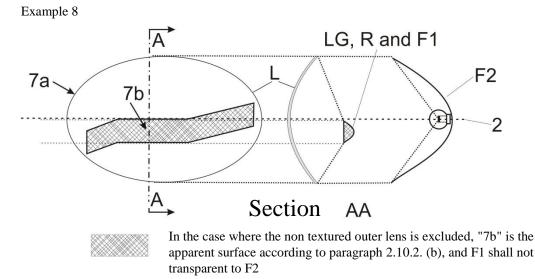
Example of a light source with a reflector optic in combination with an area which is not part of this function, behind an outer lens:
