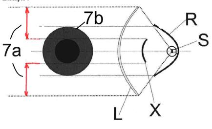
In the case where the non textured outer lens is excluded, "7b" is the apparent surface according to paragraph 2.10.2. (b).
