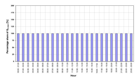
Figure 1 Daily hydrograph for feeding of on-board sewage treatment plant with upstream sewage storage tank
