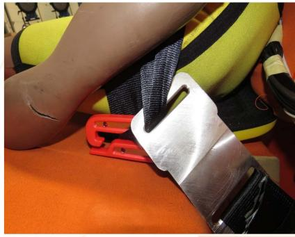
The configuration is causing narrow contact with the hip, but also contact with the webbing guide (buckle crunch!)
