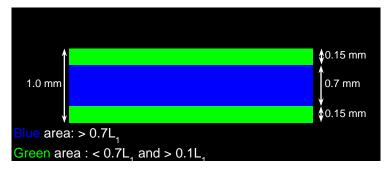
Figure 2: Luminance distribution (luminance limits) of the light-emitting-area in the worst case LED arrangement described under 3.2.
