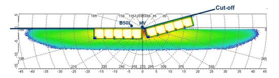
Figure 1: Relevant test points in a typical passing beam according R112, including some visualization of images of a LED light source created by reflector optics
