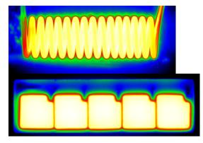
Figure 3: Luminance distribution of the light-emitting-area in case of a typical halogen bulb (left) and a typical LED arrangement for passing beam (right)
