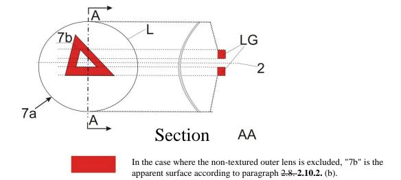
Example of a light guide optic or a reflector optic behind an outer lens:
