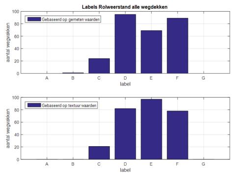
Preliminary research is possible by means of texture measurements on test sheets in the laboratory, but in the future it may also be possible to determine the rolling resistance with a sophisticated laboratory test in the laboratory (ongoing research).
