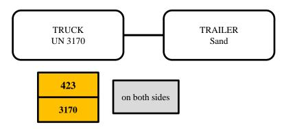
4. The other possibility – which is not in contradiction to 5.3.2.1.4, because only the transport of other dangerous goods is excluded, and the transport unit has to display the orange-coloured plates – is shown below:
