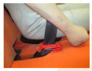
Videos will show that in the beginning of the impact the child is not held back at the pelvis and only after some time (in this case of a pure frontal sled impact) the process of holding the child at its pelvis starts effectively.
