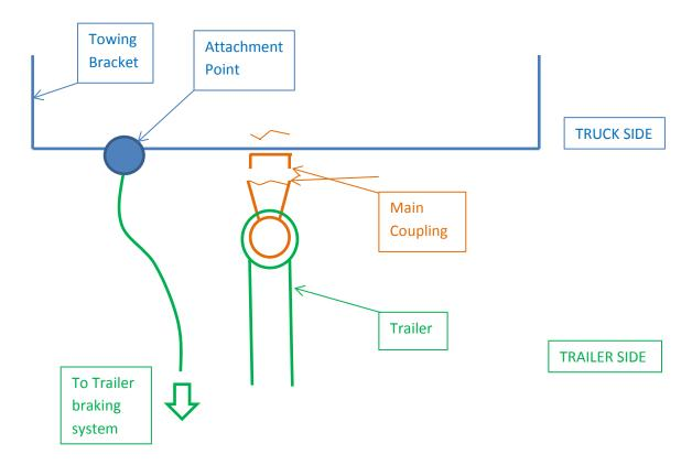
In the event of main coupling separation, the secondary device (e.g. breakaway cable) will activate the trailer brakes allowing the trailer to stop.
