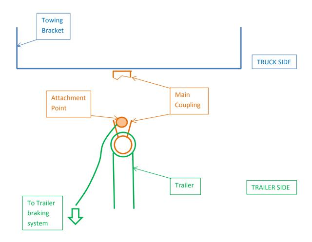
In the event of main coupling separation, the secondary device (e.g. breakaway cable) WILL NOT be able to activate the trailer brakes and the trailer WILL NOT stop.
