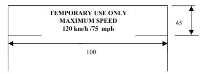
Upper case letters shall be at least 5 mm high and the numbers "120" and "75" shall be at least 20 mm high with the elements that make up each character of the number at least 3 mm line thickness. Lower case text shall at least have a line height of 5 mm. All text shall be enclosed in a border and be on a background of contrasting colour.
