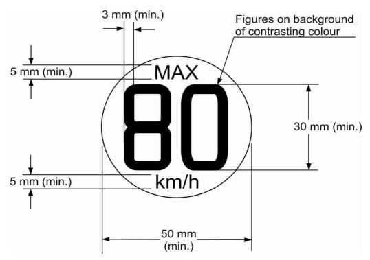
In the case of vehicles intended to be sold in countries using imperial units of measurement, an additional warning symbol, identical to that described above, with the exception that the figure "80" shall be replaced by "50" and the wording "km/h" by "mph", shall be permanently displayed on the outer face of the wheel in a prominent position.
