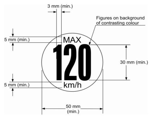
In the case of vehicles intended to be sold in countries using imperial units of measurement, an additional warning symbol, identical to that described above, with the exception that the figure "120" shall be replaced by "75" and the wording "km/h" by "mph", shall be permanently displayed on the outer face of the wheel in a prominent position.
