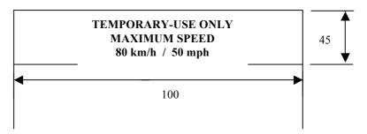
Upper case letters shall be at least 5 mm high and the numbers "80" and "50" shall be at least 20 mm high with the elements that make up each character of the number at least 3 mm line thickness. Lower case text shall at least have a line height of 5 mm. All text shall be enclosed in a border and be on a background of contrasting colour.
