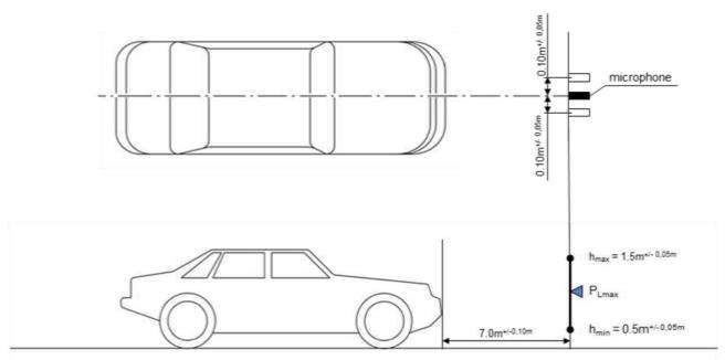
$\begin{array}{ll} h_{\text{min}} & \text{minimum height for measurements} \\ h_{\text{max}} & \text{maximum height for measurements} \\ P_{\text{Lmax}} & \text{Point of maximum sound pressure level} \end{array}$
