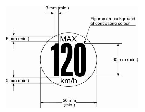
In the case of vehicles intended to be sold in countries using imperial units of measurement, an additional warning symbol, identical to that described above, with the exception that the figure "120" shall be replaced by "75" and the
