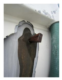
The dark grey area with the plug is the protective lining, the light grey colour is the aluminium alloy shell material and the peeling off white/grey is the paint.
