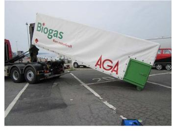
A MEGC being unloaded from a truck by the hooklift hoist
