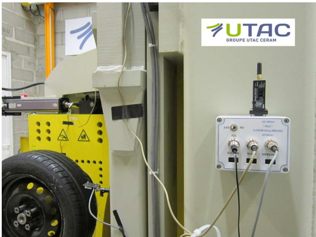
Figure 2. Installation of NAMI-357 data logger on MTS test machine in UTAC.
