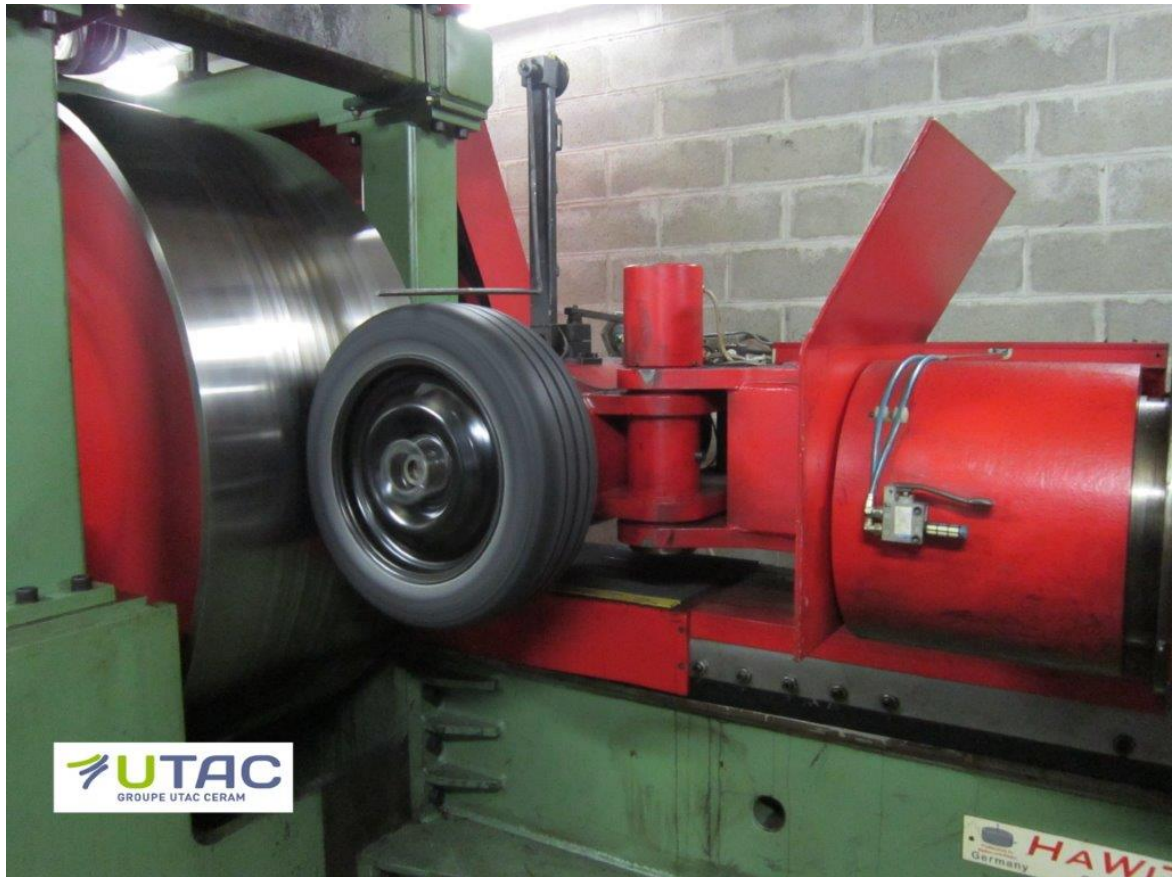
Figure 5. View on HAWITEC test machine in UTAC on which NAMI-357 data logger and drum sensors “S” were used
