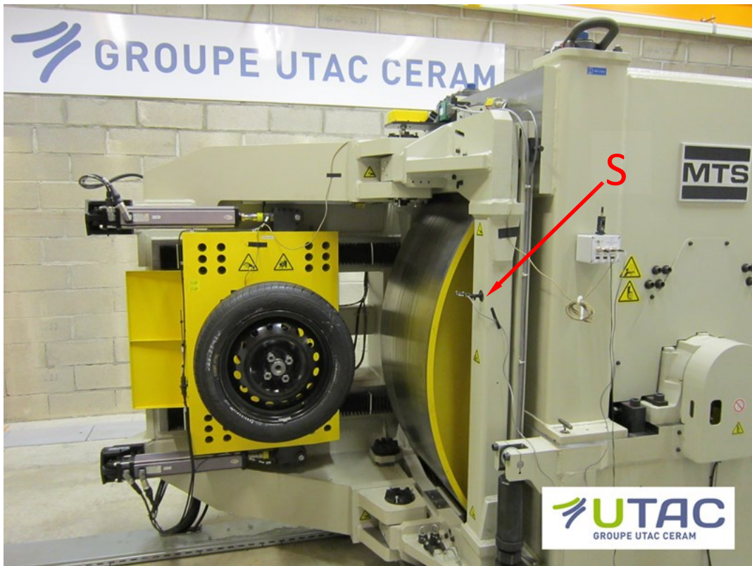
Figure 3. NAMI-357 data logger and drum sensors “S” view on MTS test machine in UTAC.
