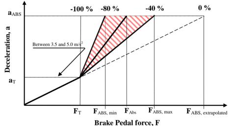
8.2.4. A straight line is drawn from the origin through the point  $F_T$ ,  $a_T$  (as shown in Figure 1a). The value of brake pedal force "F", at the point of intersection between this line and a horizontal line defined by  $a=a_{ABS}$ , is defined as  $F_{ABS, extrapolated}$ :
