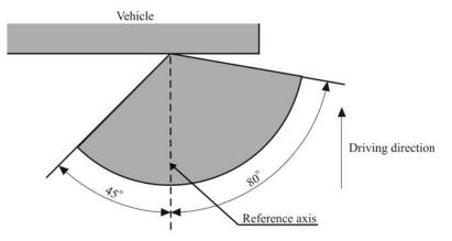
However, in the case where a device is intended to be installed with its H plane at a mounting height less than 750 mm above the ground, the inward angle of  $45^{\circ}$  may be reduced to  $20^{\circ}$  under the H plane."
