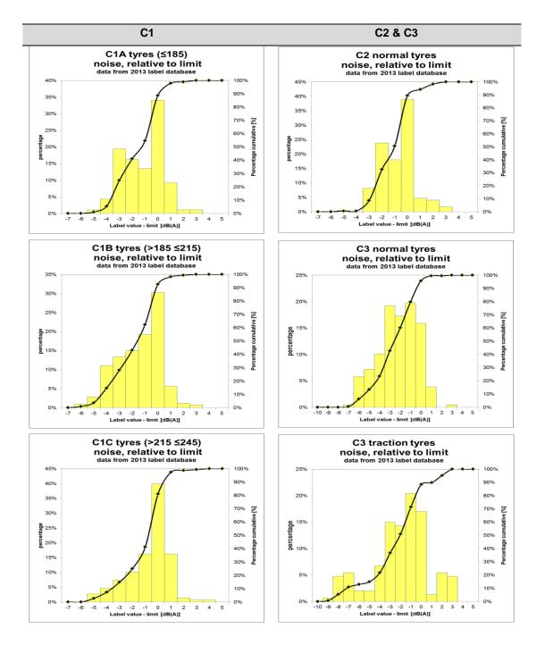
figure 3 Statistical distribution of tyre noise emission values relative to the limit. The limits may consist of the sum of the base limit plus a margin for special properties (snow use etc) if relevant.
