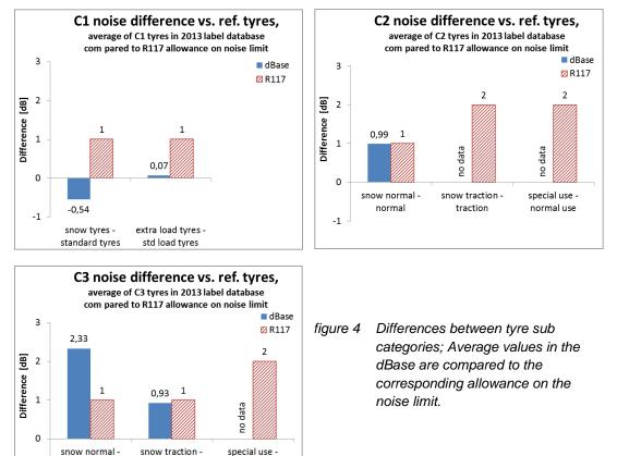
For C1 tyres the +1 dB correction for snow tyres and extra load tyres overestimates the actual effect of such specific characteristics observed in the 2013 data set. Snow tyres were found to exhibit about 0.5 dB lower values compared to standard tyres. Extra load tyres have an almost equal level compared to standard load tyres.
