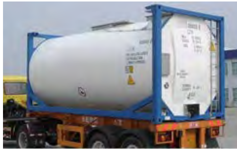
Figure 3.41 25,000 l collar tank
