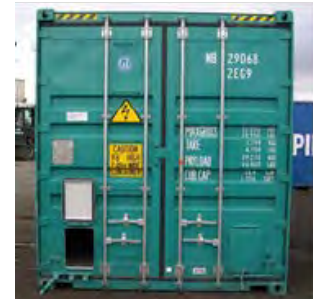
Figure 3.45 Cat flap type hatch in rear doors
