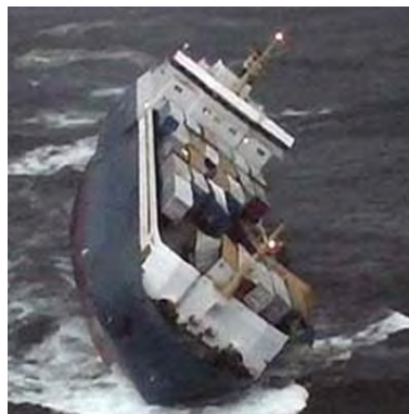
Figure 1.5 Heavily listing vessel after cargo has shifted
