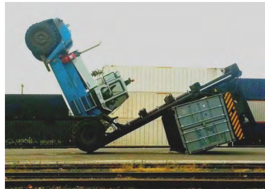
Figure 1.14 Tipped container handler (© abc.net.au)
