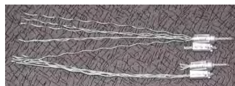
Figure 9.27 Cut cable seals
