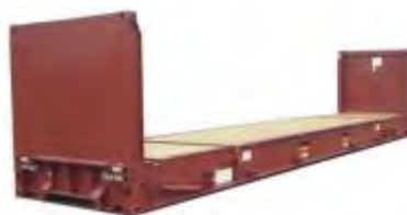
Figure 3.50 40-foot folding flatrack
