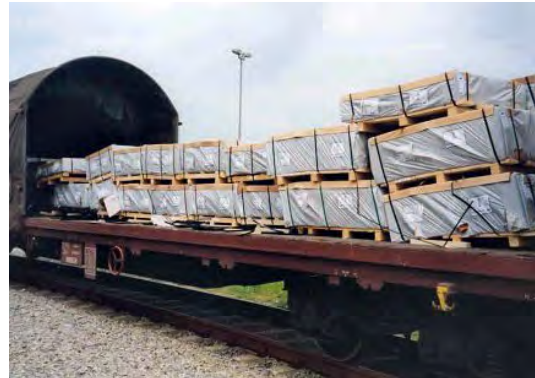
Figure 1.7 Loose packages on rail wagon
