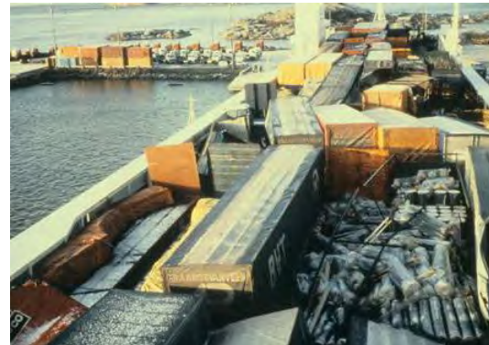
Figure 1.4 Shifted cargo on a RO/RO deck
