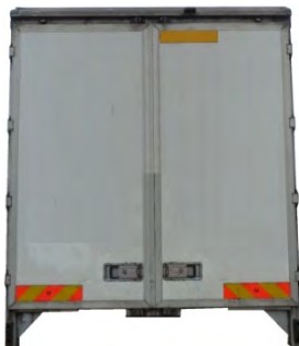
Figure 9.2 Swing door (Road vehicle)
