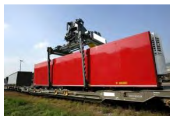
Figure 3.87 Trailer1 loading using grapple arms
