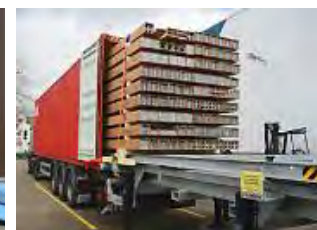
Figure 3.10 Unit load packing
