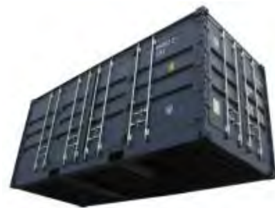
Figure 3.27 20-foot side door container
