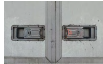
Figure 9.7 Recessed handles with protruding eyes
