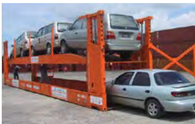
Figure 3.54 45-foot car carrying folding flatrack
