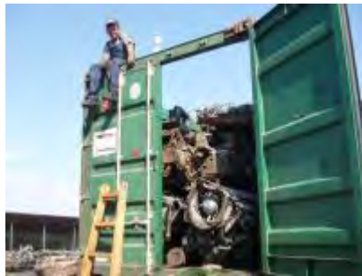
Figure 3.22 20-foot open top with scrap steel
