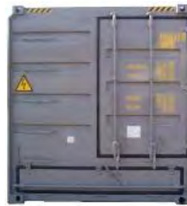
Figure 3.44 letterbox type hatch in fixed rear end
