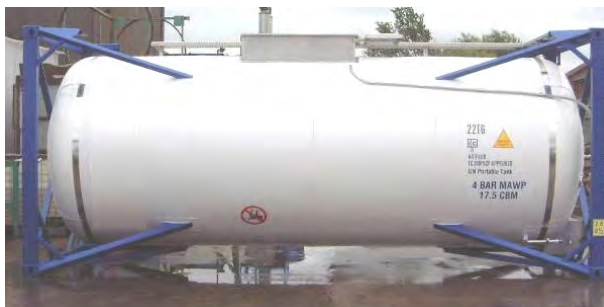
Figure 3.38 Beam tank no top rail
