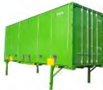
Figure 3.67 Class C side door swap body
