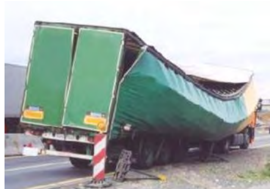
Figure 1.2 Inadequate side wall strength
