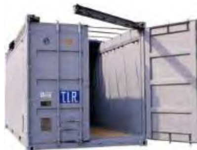
Figure 3.21 20-foot open top with tilt removed and rear header open
