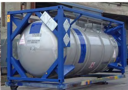
Figure 3.39 Beam tank with top rail
