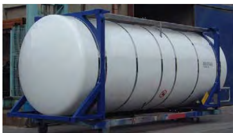
Figure 3.68 Swap tank showing exposed ends
