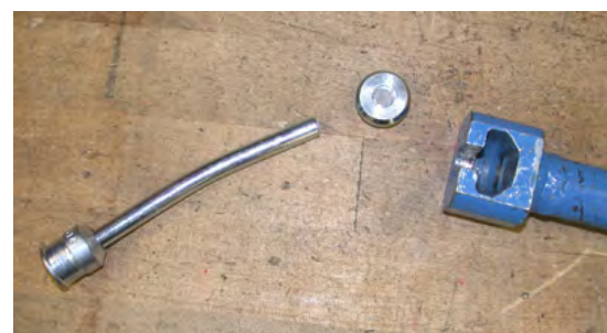
Figure 9.33 Rail car bolt seal and breaking tool
