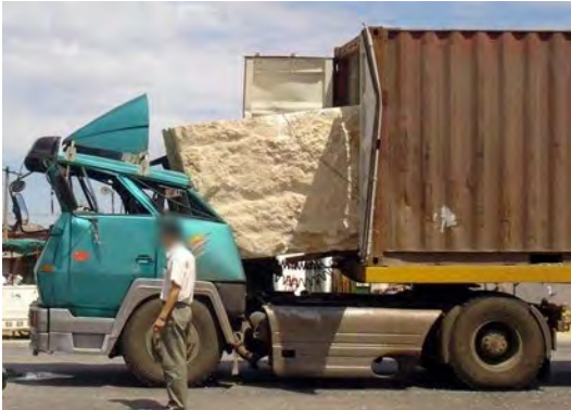
Figure 1.1 Lack of longitudinal securing
