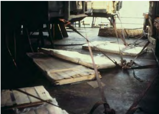
Figure 1.3 Cargo breaking out of a trailer
