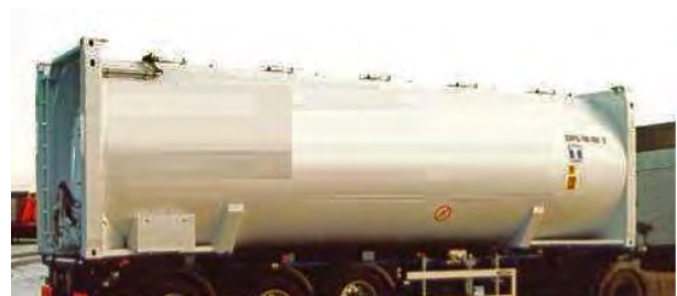
Figure 3.69 30-foot stackable swap tank for powder
