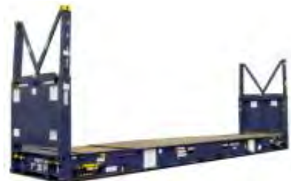
Figure 3.51 40-foot folding super rack
