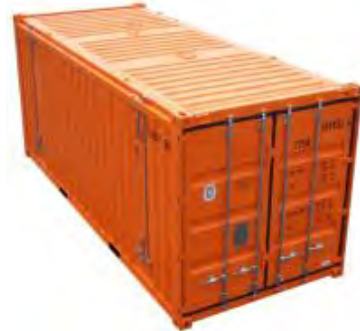
Figure 3.20 20-foot open hard top container
