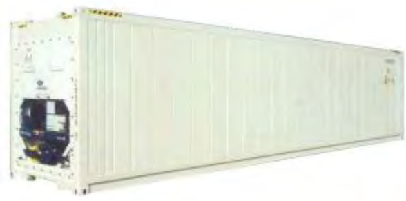
Figure 3.34 40-foot refrigerated container
