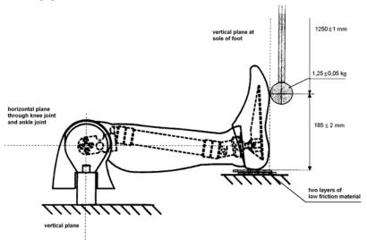
Figure 2 Lower foot impact test (without shoe)
