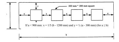
Figure 3 Honeycomb axes and measured dimensions
