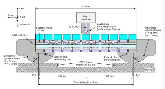
$F_c$ : External loading force at center of the tibia  $D_c$ : Deflection at center of the tibia  $M_c$ : Moment Center (Nm) =  $F_c/2$  (N) x 0.205 (m) R: Radius, W: Width along to the side axis Tolerances for all dimensions above:  $\pm 2$  mm
