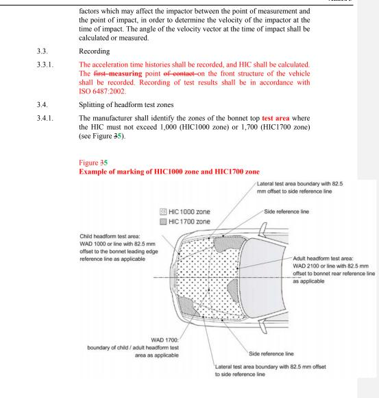
3.4.2. Marking of the "bonnet top" **test area** impact area as well as "HIC1000 zone" and "HIC1700 zone" will be based on a drawing supplied by the manufacturer, when viewed from a horizontal plane above the vehicle that is parallel to the vehicle horizontal zero plane. A sufficient number of x and y co-ordinates shall be supplied by the manufacturer to mark up the areas on the actual vehicle while considering the vehicle outer contour in the z direction.
