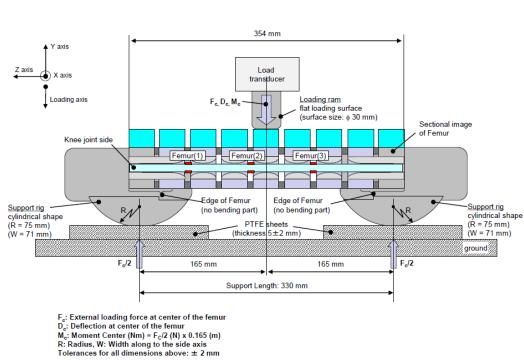
Flexible lower legform: Impactor test set-up for the femur in the static certification test (see paragraph 1.2.4. of this Annex)
