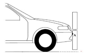
$<sup>^2</sup>$  Remark: due to the spatial geometry of the bonnet top, the first contact may not occur in the same vertical longitudinal or transverse plane which contains measuring point A.
