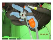
Load can be applied without any interference between the device and the harness.
