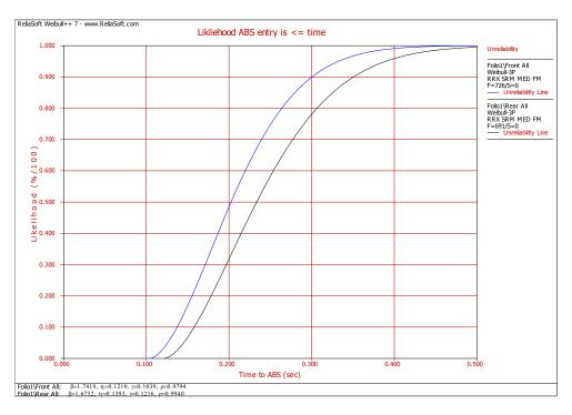
By reducing the lower limit to 0.1 seconds the test failure rate reduces to practically zero. Allowing the reduction tends to make the regulation more stringent by including a greater number of brake force application rates and eliminates restrictive test requirements.
