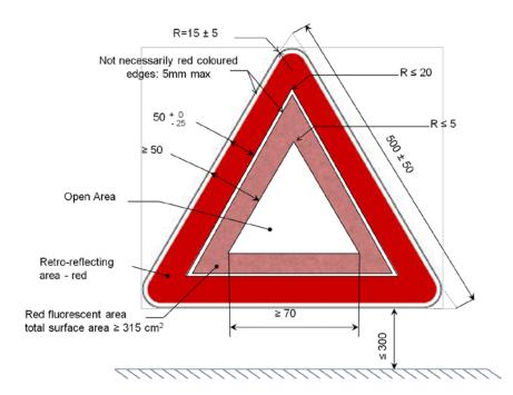
"Figure 2 Shape and dimensions of the advance-warning triangle of type 2 and of the support  $\,$
