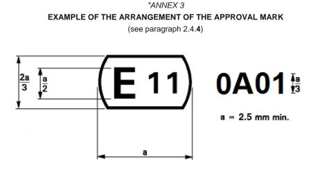
The above approval mark affixed to a gas-discharge light source indicates that the light source has been approved in the United Kingdom (E11) under the approval code 0A01. The first character of the approval code indicates that the approval was granted in accordance with the requirements of Regulation No. 99 in its original form."
