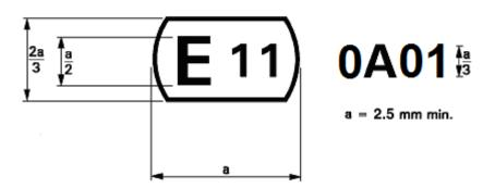
The above approval mark affixed to a LED light source indicates that the light source has been approved in the United Kingdom (E11) under the approval code 0A01. The first character of the approval code indicates that the approval was granted in accordance with the requirements of Regulation No. 128\* in its original form."
