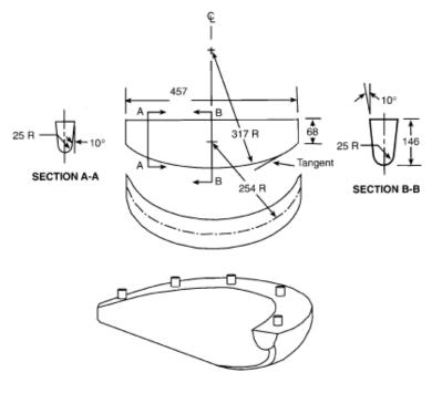
MATERIAL: Cast Aluminum 355 T-6 Condition Finish-1.3 Micrometer (um)
