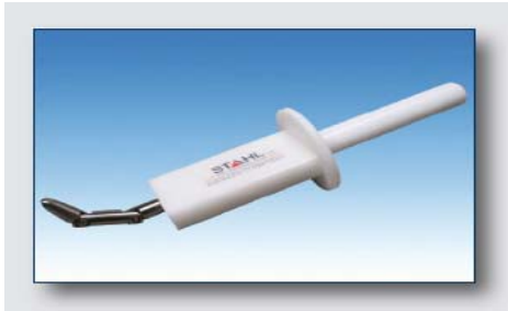
Figure 6 Standardized Test Finger
