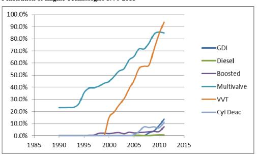
Figure 3 Penetration of Engine Technologies 1990-2011<sup>25</sup>
