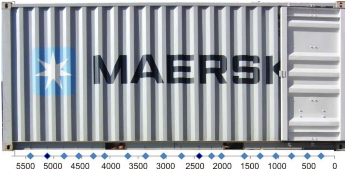
Distance of cross members from door bottom corner castings (outer surface) to the centre of cross member
