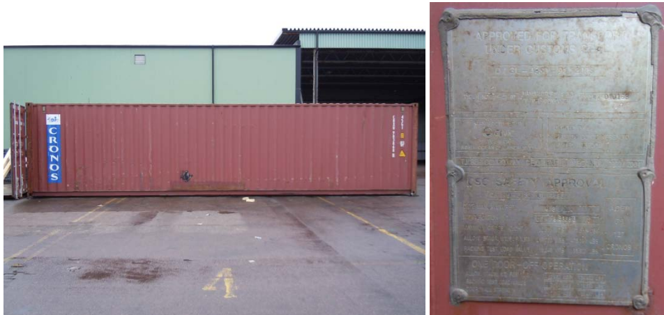
40' CRONOS container 45G1 (CRXU 983868-8) used in tests in Helsingborg with a payload of 28.6 ton.
