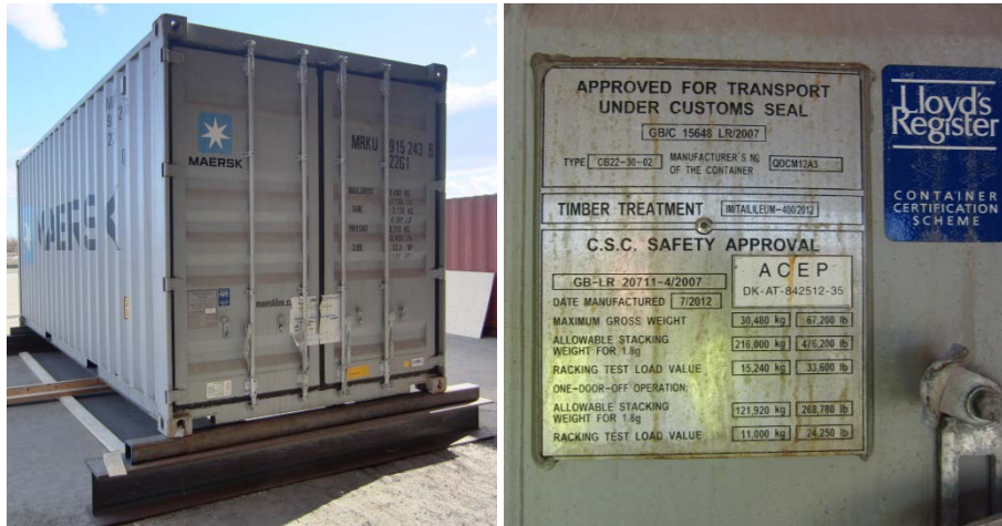
20' MAERSK container 22G1 (MRKU 915243-5) used in tests in Avesta with a payload of 28.3 ton.
