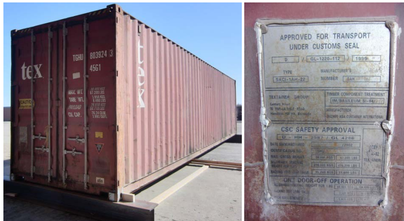
40' TEXTAINER container 45G1 (TGHU 803924-3) used in tests in Avesta with a payload of 26.6 ton.
