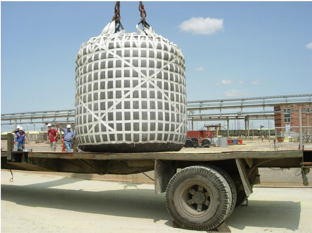
FBC was freely mounted on the truck platform. Tilting of platform with FBC and overturning prevention measures were carried out by 2 crane trucks of relevant capacity. The tilting angle was controlled by a digital inclinometer BOSH “DNM 60L”. All testing procedure was shot by the photo/video camera CASIO Exilim “EX FH -100”.
