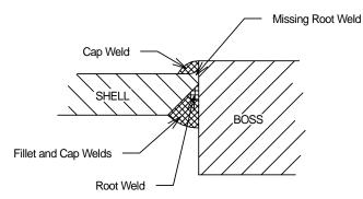
This missing weld gave an indication, during the magnetic particle inspection, that an internal crack was present along the length of the missing weld.
