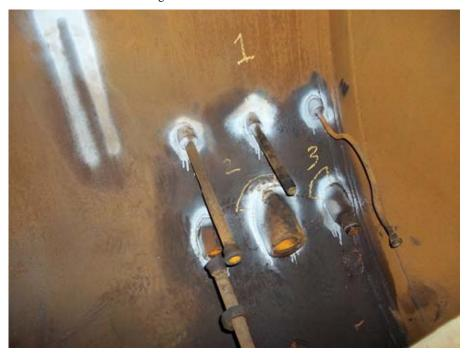
17. Following the initial indications of cracking light grinding of the surface was undertaken to ensure that it was not just weld overlap, however it was confirmed that all three were hairline cracks (the white background paint and black indicator has now made these very visible to the naked eye).
