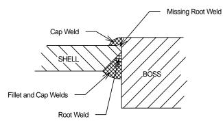
This missing weld gave an indication, during the MPI examination, that an internal crack was present along the length of the missing weld.
