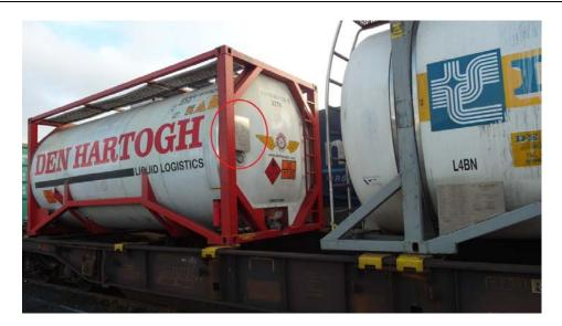
7. On this tank-container the metal plate is located in the red circle.
