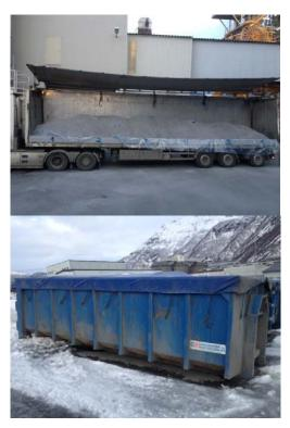
A sheeted semitrailer and a sheeted container loaded with UN3170
