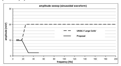
6. The test duration is also aligned with UN38.3, Test T3, requiring 12 transitions from the minimum to the maximum frequency and back within 15 min., resulting in a total test duration of 3 hours.
