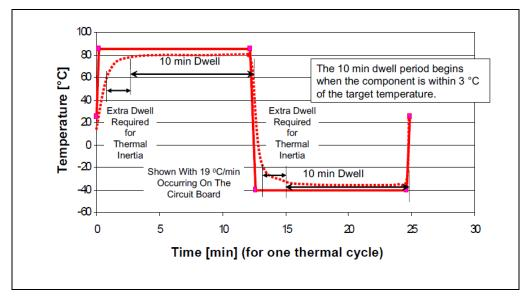
18. Since the REESS has a different thermal mass and has different operation and storage temperature ranges than typical electric / electronic components, a modification of the test conditions i.e. lower maximum temperature and longer dwell time are needed.
