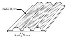
Dimension of the crush plate: 600 mm x 600 mm or smaller
