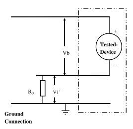
If V2 is greater than V1, insert a standard known resistance (Ro) between the positive pole of the Tested-Device and the ground connection. With Ro installed, measure the voltage (V2') between the positive pole of the Tested-Device and the ground connection (see Figure 3).
