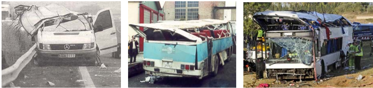
Figure 1. Collapsed superstructures in bus rollover
