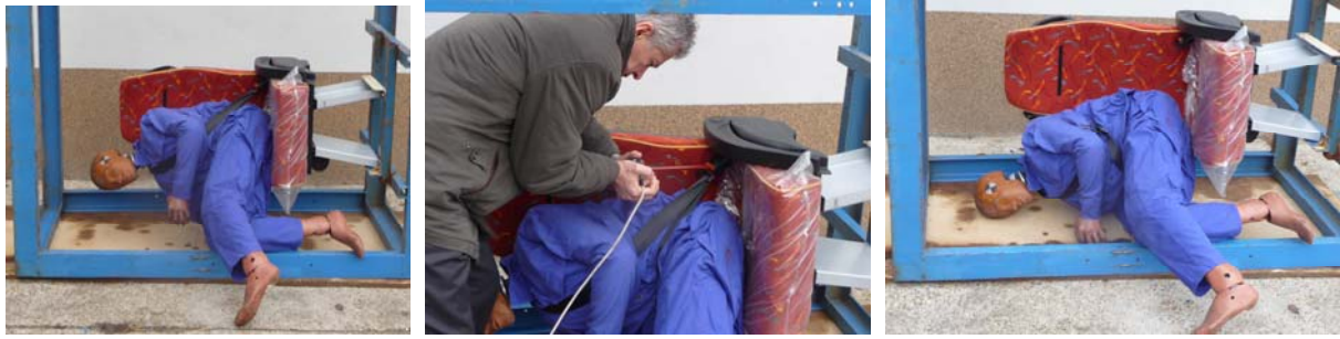
Figure 8. Hanging dummy, 3 pts belt – no way to release the safety belt
