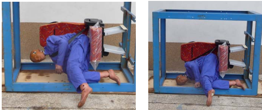
Figure 9. 3 pts and 2 pts belted dummies in final position
