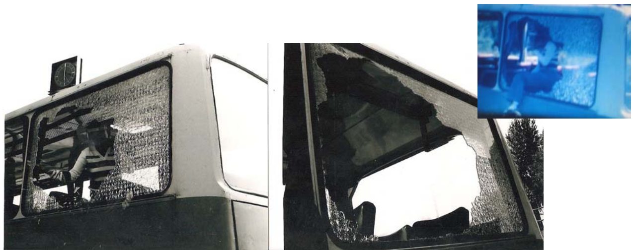
Figure 16. Arrangement of evacuation test through side window
