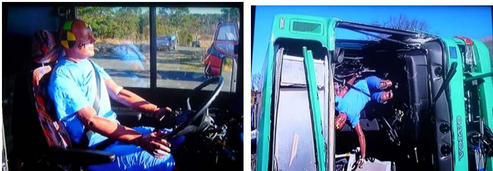
Figure 11. Original and final position of the “driver” in the VOLVO rollover test.
