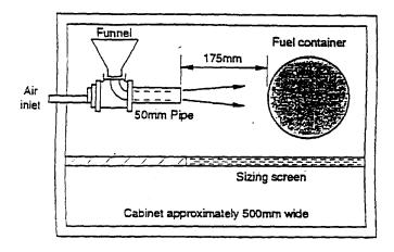
Figure H.2 - Gravel impact test
