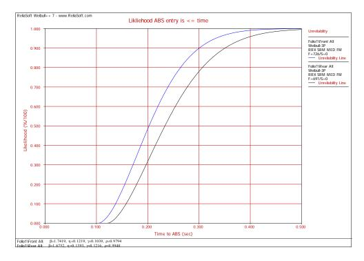
By reducing the lower limit to 0.1 seconds the test failure rate reduces to practically zero. Allowing the reduction tends to make the regulation more stringent by including a greater number of brake force application rates and eliminates restrictive test requirements.
